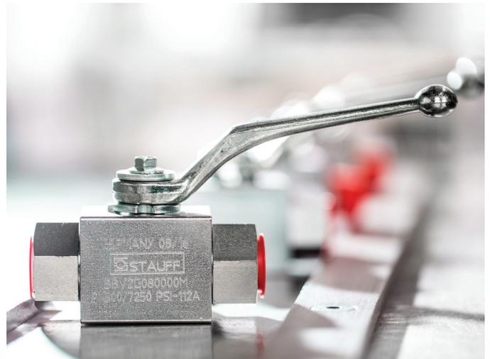
The established zinc/nickel surface offers over 1,200 hours of resistance to red rust/base metal corrosion under practical test conditions in the salt spray chamber in accordance with EN ISO 9227. The chromium(VI)-free coating exceeds the highest requirements with regard to durability, as defined in the VDMA Standard Sheet 24576. It has a high-quality appearance similar to stainless steel, while complying with all relevant ELV, REACH and RoHS guidelines.
